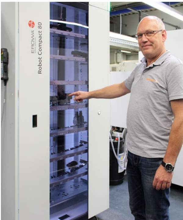
Fig. 3: Ralf Runte, Group Leader Mechanical Processing Tooling at Weidmüller: „We have combined an EROWA ERC 80 robot with an ATOS ScanBox Series 4 from GOM into an automation solution.“
