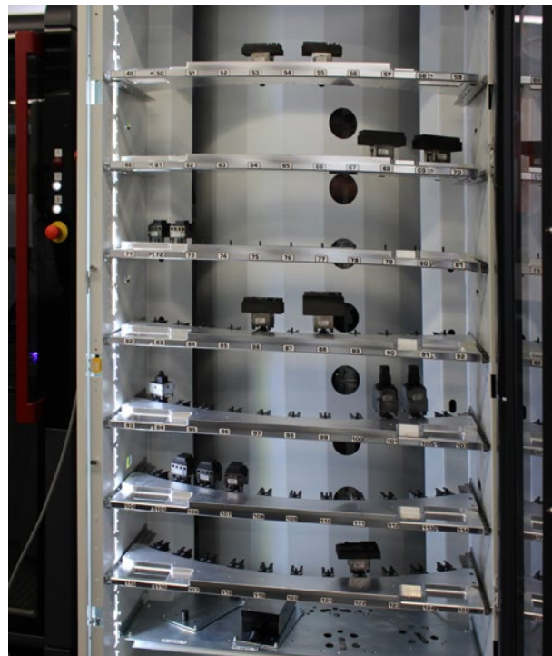
Fig. 4: Up to 120 electrodes can fit in the system's magazine
