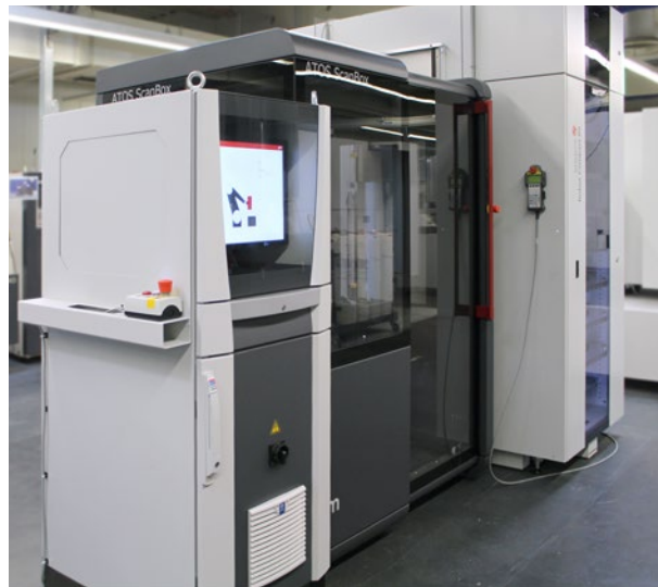
Fig. 2: The electrodes sit on mounts which have chips that the CERTA software uses to control and monitor the robot, the pallet changer and the entire handling process for substituting the parts into the ATOS ScanBox
